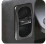
COMPRESSOR SWITCH/AIR RELEASE VALVE
